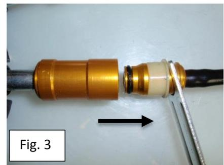
The new clip style connector, Fig. 5 only requires removing the clip. A small flat screwdriver or needle nose pliers can be used to remove the clip, and the line will pop out, Fig. 6.
