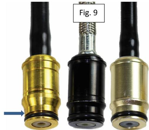
Fig. 9 L-R shows a gold or brass color, black color and a non-standard color produced by an aftermarket supplier. By color the one on the right is not gold or brass but by dimensions and profile it is the black connection. The manufacturer has not maintained the precedent of the gold or brass color vs. black to provide visual confirmation. The sleeves were removed to aid in illustrating the color of the plug.
