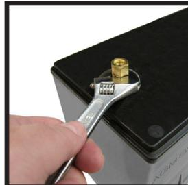
Always make sure to tighten your brass adapters after you have hand tightened them. This will give you a connection that won't loosen while you are working with the battery. Giving you the best and most consistent test and charge.
