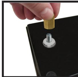
Clean the threaded steel post and its lead pad base to make sure you get the best connection possible. One of the great features of the AutoMeter Group 31 brass adapters is they can cut through corrosion that may have collected at the base of the terminal.
