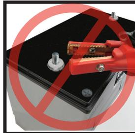
Never connect directly to the steel threaded posts when charging or testing your battery since it will produce false readings due to the high resistance of the steel. You also shouldn't connect directly to the steel threaded posts when charging because it can lead to severe battery and clamp damage.
