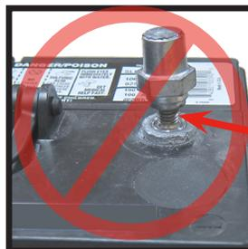
Adapter **MUST** make contact with Lead Pad at bottom.
