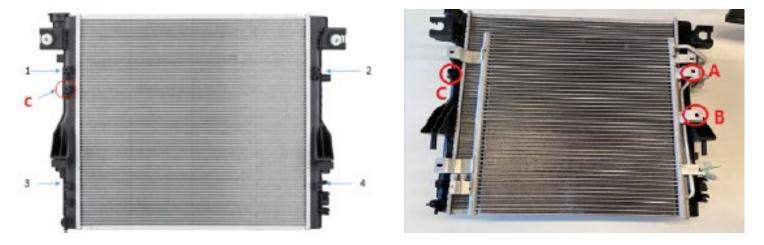
The pictures display the radiator with numbered mounting points the correspond to the condenser. As well as lettered points corresponding to auxiliary oil cooler mounting on both the condenser and radiator. The radiator/condenser pairing is what makes up the auxiliary oil cooler mounting
